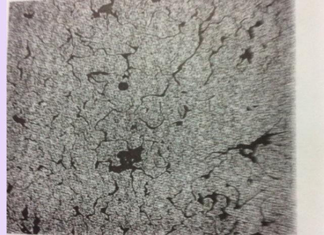
FIGURE 4.14 Flake Graphite Typical of Magnesium-Treated Iron Contaminated with Lead (0.0086%) and Antimony (0.0057%) (100x, Unetched).
